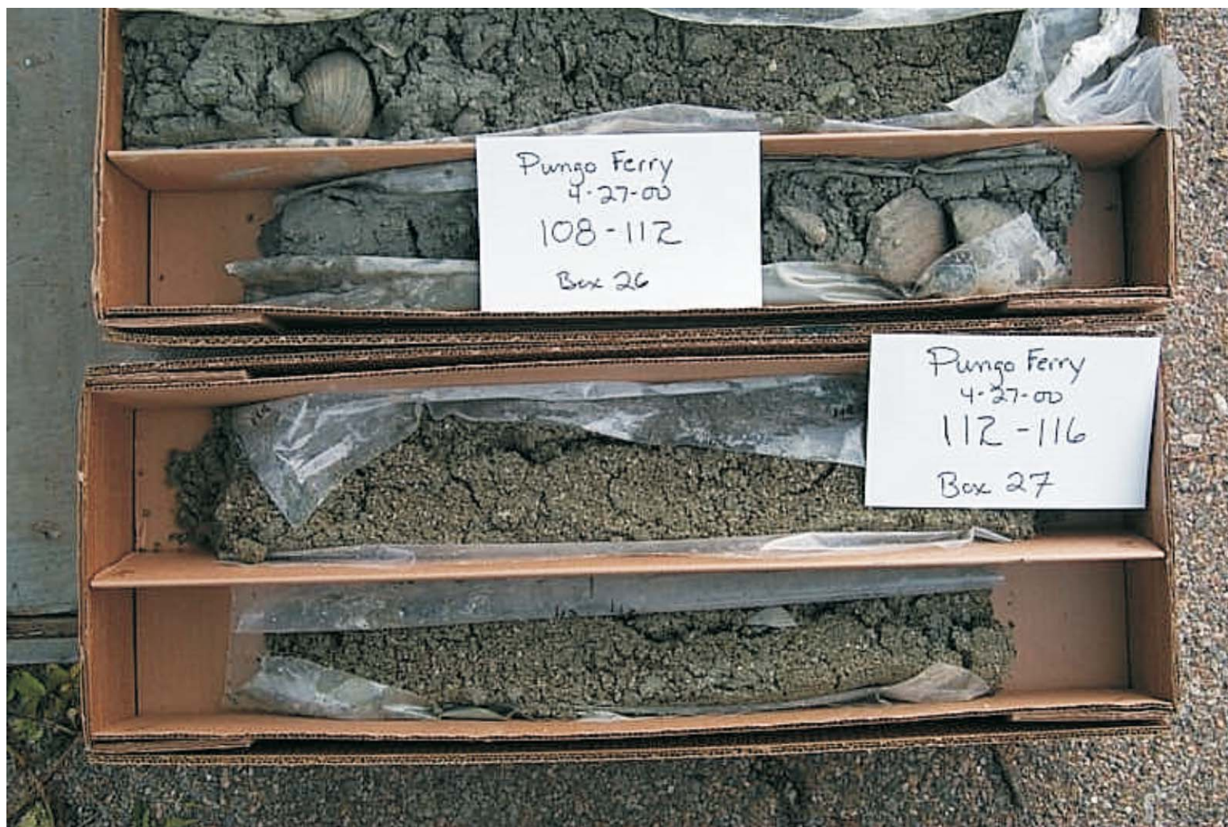
Figure 4. Core samples of the Yorktown confining unit (Box 26) and the Yorktown-Eastover aquifer (Box 27) from Old Pungo Ferry Road site, Virginia Beach, Virginia.
