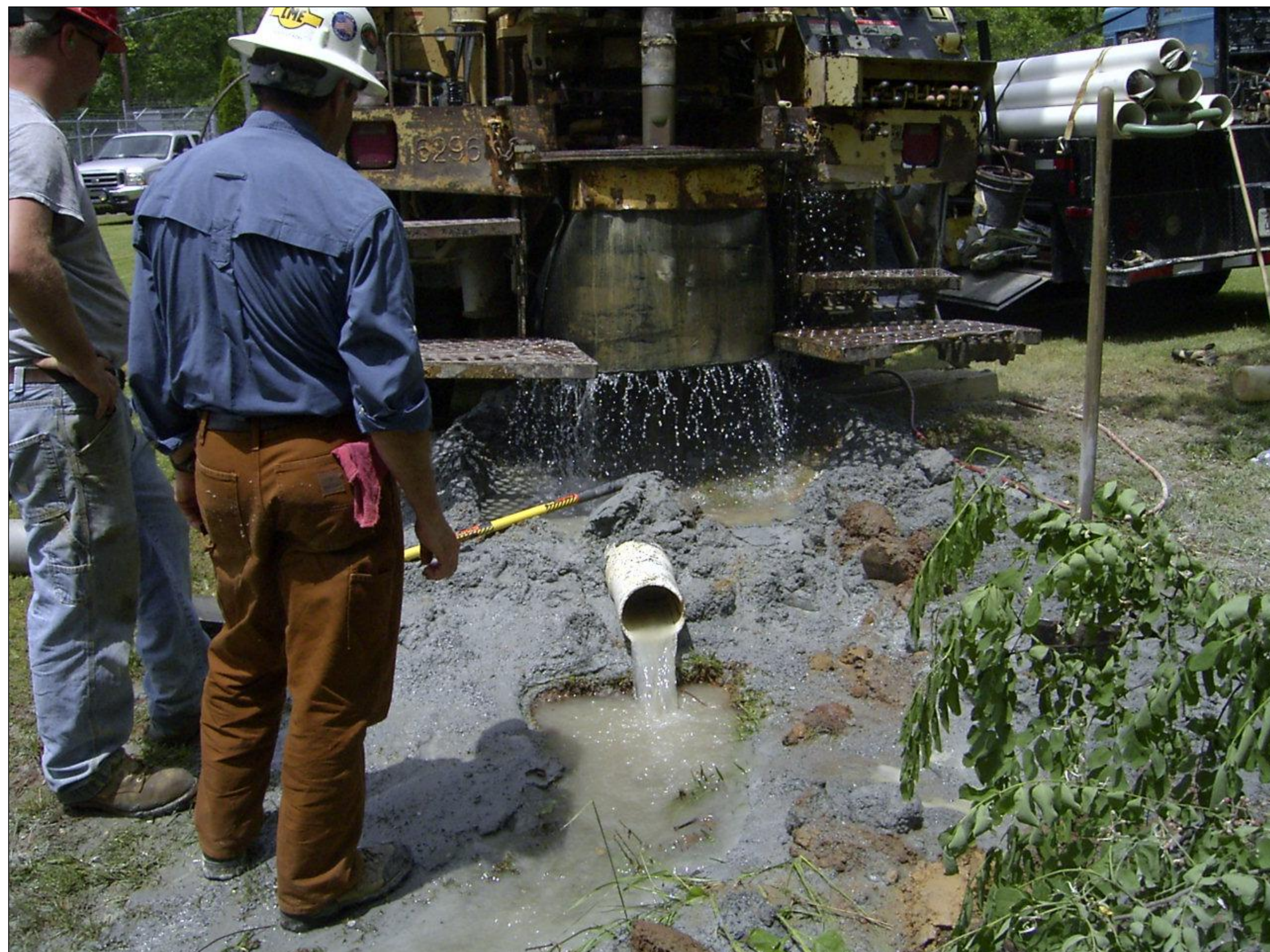
Figure 2: DEQ staff and Bedford Well Drilling evaluate the yield of Otterville SOW 226 during an air-lift test shortly after completion. The well was completed in Proterozoic granitic gneiss (Suck Mountain Pluton) estimated yield during air-lift test was 60 gal/min.
