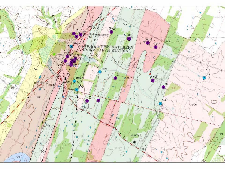
**Preliminary Findings of Drilling Phase of Project** Locating potential high yielding wells was easier than originally anticipated. There is good correlation between well yield hand discharge areas, geologic structure, and locations of faults. Surface geophysical surveys show great promise as a potential prospecting tool and high conductivity zones correlate with geologic structure and faults
