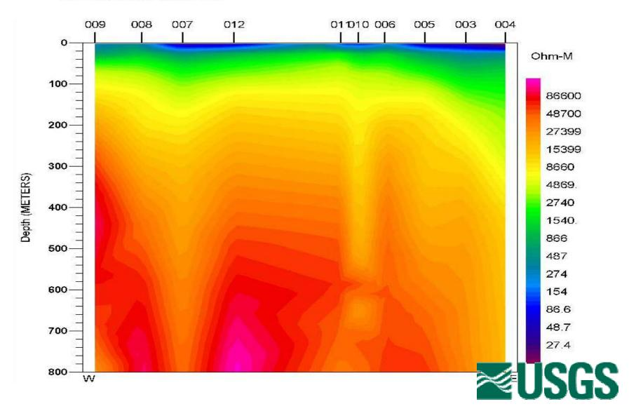
**Preliminary Findings of Drilling Phase of Project - Continued**  Upper portion of aquifer is highly permeable, filled with solution yoids, and has the capacity yield large quantities of water. This zone is characterized by large solution voids, many of which are clay filled. Water quality of these zones would likely be subject to contamination and may have problems with turbidity. **ZUSGS**
